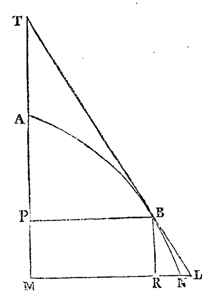
Let AB be a Curve, the Abscisse AP = x, the ordinate PB = y, the Difference of the Abscisse PM = dx, the Difference of the Ordinate RN = dy. Now by supposing the Curve to be a Polygon, and consequently BN, the Increment or Difference of the Curve, to be a straight Line coincident with
